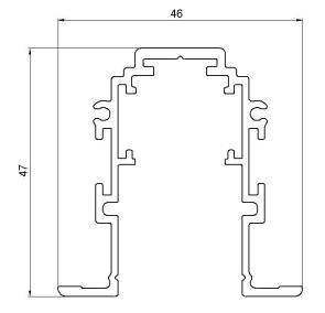
Dimensions: 4000 x 47 x 46 mm Max voltage: 48 V, 10 A Max wattage: 200 W Weight: 4 kg
